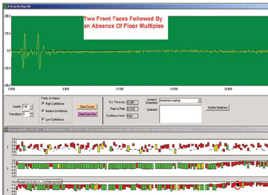
This analyst display shows the A-scan UT image of a coating failure. UT scanning is required unless the tank environment is clear enough to allow direct visual inspection (Fig. 5).
