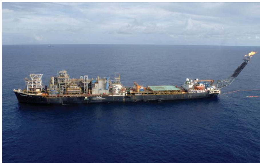
Petrobras, in September 2008, started a long-term production test of a subsea completed presalt well in the Jubarte field, off Brazil. The presalt 30° oil flows to the P-34 floating production, storage, and offloading vessel that also processes production from wells completed in a Jubarte heavy oil reservoir above the salt layer. Photo from Petrobras.
